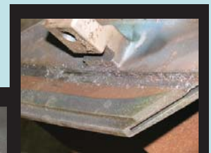
Material deposit on nozzle
